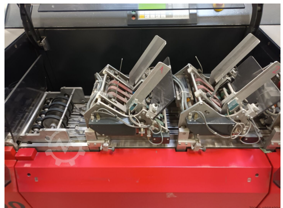
A Kern 3000 from the 1980s. These were complex electro-mechanical devices for inserting printed matter into envelopes. (c) source
